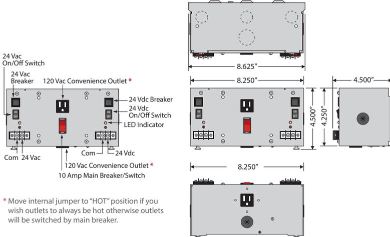
\* Move internal jumper to "HOT" position if you wish outlets to always be hot otherwise outlets will be switched by main breaker.
